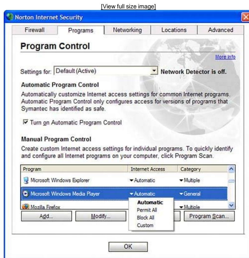
Figure 10.1. Norton Personal Firewall allows users to define permitted and denied activity for specific applications.
