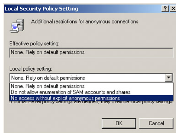
Figure 9.2. You can limit null session connections by restricting anonymous actions using the Local Security Policy editor or through Group Policy.
