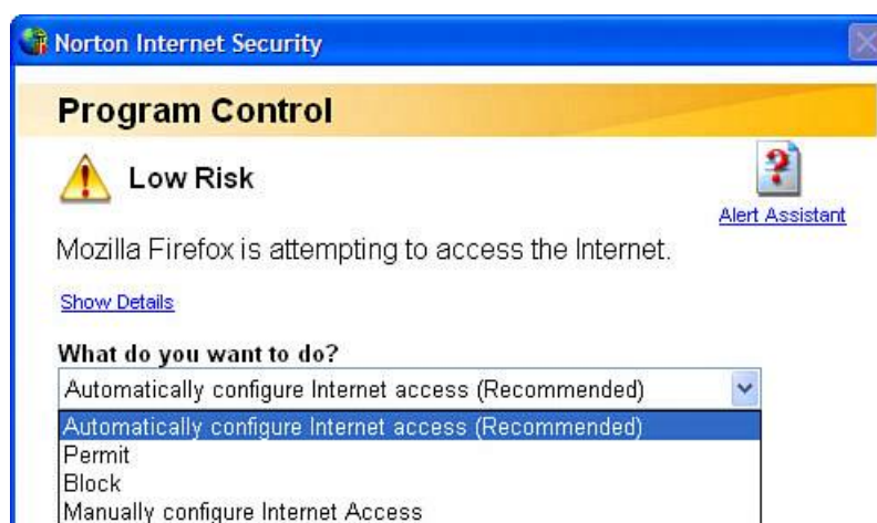
Figure 10.4. Norton Personal Firewall can be configured to prompt the user if an unfamiliar application attempts to initiate a network connection.
